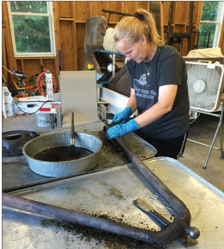
Judy Dann chips away at 88 years of grease and grime on the front radius rod of Velma. Some day this radius rod will look like new. (Rich Dann)
